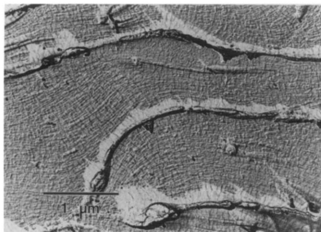
Figure 3 TEM micrograph of a two-stage replica of a film etched in 1 wt% \text{KMnO}_4 solution in 2:2:1 \text{H}_2\text{O}:\text{H}_3\text{PO}_4:\text{H}_2\text{SO}_4 for 3 h at 30^\circ\text{C} . Both lamellae and fibrils are revealed
